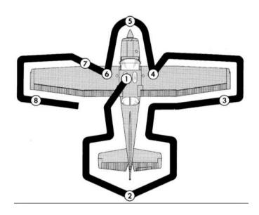
Visually check airplane for general condition during walk-around inspection.
