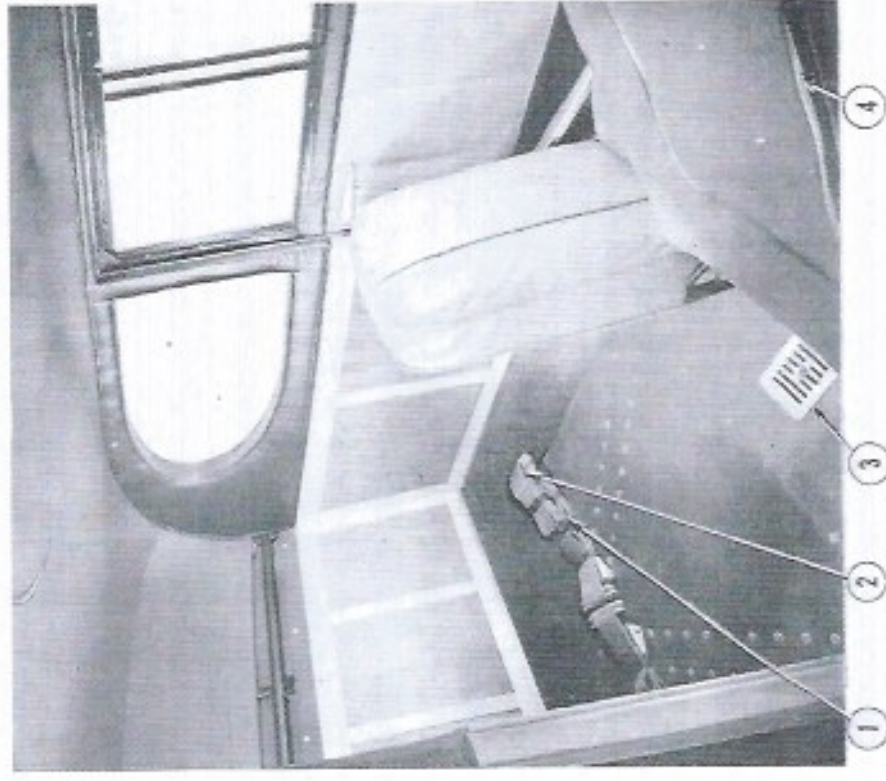
1. Rear Safety Belts 2. Cargo Retainer Straps 3. Rear Heater Port 4. Map Pocket
