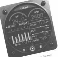
this screen is displayed on power-up and is the screen that should be monitored for most of the flight. Buttons and Knob operate as follows: (S)creens Button - Switches the display between the various screens.
